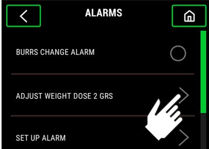
**10.12.4.** Change the grams of Dose 2 by sliding the grams or tenths of a gram up or down until the desired weight is reached and press the button **OK** to accept.
