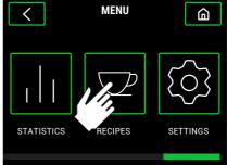
**10.6.2** There are two options, the first one will access the menu to configure the dose times, the second will activate or deactivate the Grinding Pause (by default it is active).
