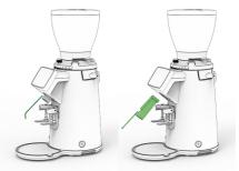
**11.3.2.** For the **E10**, to properly disassemble the regulator, please follow the steps outlined in section **12.3.7.** for standard grinders or section **12.3.10.** for grinders equipped with the **Lock Load System**. Use the #3 Hex Allen key supplied to loosen the screw that holds the nozzle located on top of the grinding cavity, according to (**Fig. 1**), and remove it by pulling downwards, as shown in (**Fig. 2**).
