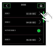
**10.2.3.** Inside the dose time configuration menu, this can be changed by sliding the seconds and tenths of a second up or down until the desired time is obtained and press **OK**.
