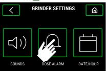
**10.12.2.** Activate or deactivate the Burrs change alarm by pressing **•**, adjust the Weight of the Dose 2, the Burrs change alarm Kg or Reset Alarm.
