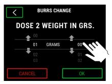
**10.12.5.** To delete the stored data of the Burr change alarm, i.e. once replaced the current set of Burrs, scroll vertically, press the Reset Alarm button and then enter the Password.
