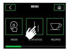
**10.5.2.** The number of independent doses for each selection is shown, either absolute which is from the date of installation of the grinder, or relative from a counter reset date. Burrs wear can also be checked here.
